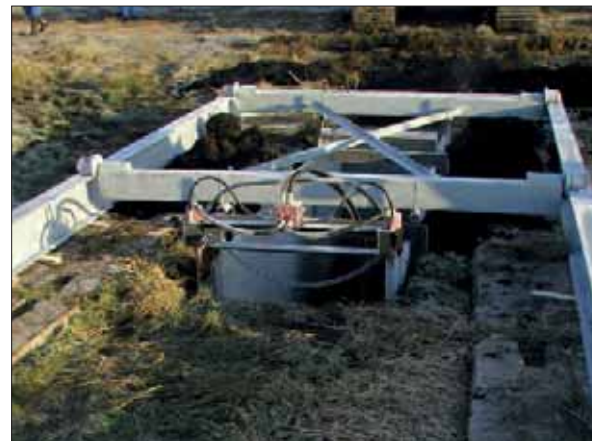
Lysimeter vessel in starting pit
