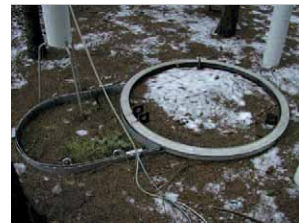
High grade steel lysimeter with planted hatch
