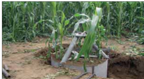
Cutting of a soil monolith in the maize field
