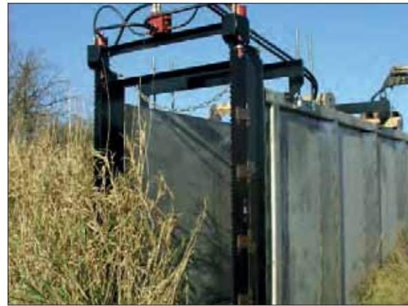
Fen lysimeter vessel with monolith cutting tools
