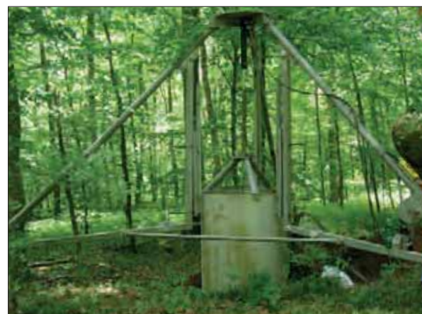
Cutting the lysimeters in a forest stand, only possible because of the easy moveable UGT technology
