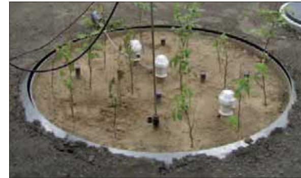
Root studying with rhizotrons and microcameras
