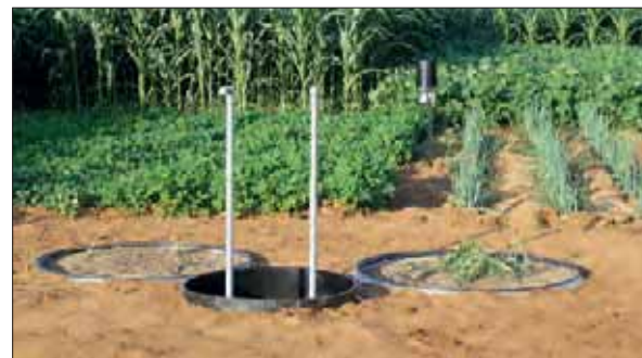
View of the newly installed lysimeter station at the Miyun reservoir
