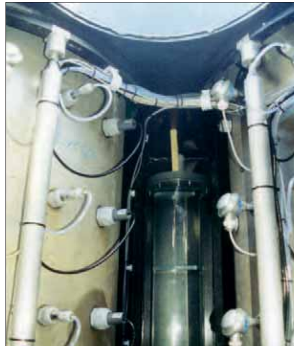
Tensiometers equipped to monitor the matric potential in the whole soil column
