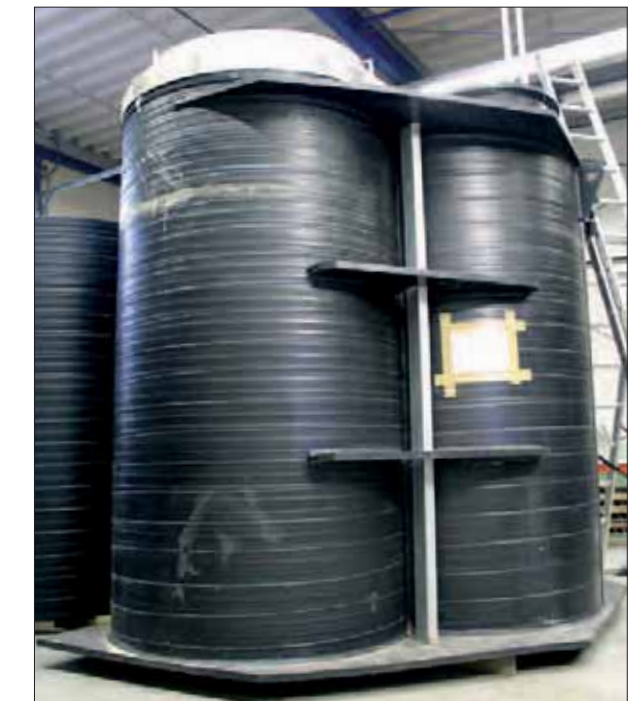
Lysimeter station under construction
