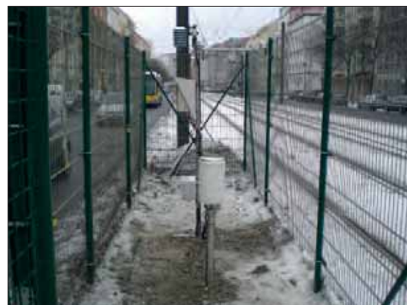
Embedded platy lysimeter and meteorological measuring station
