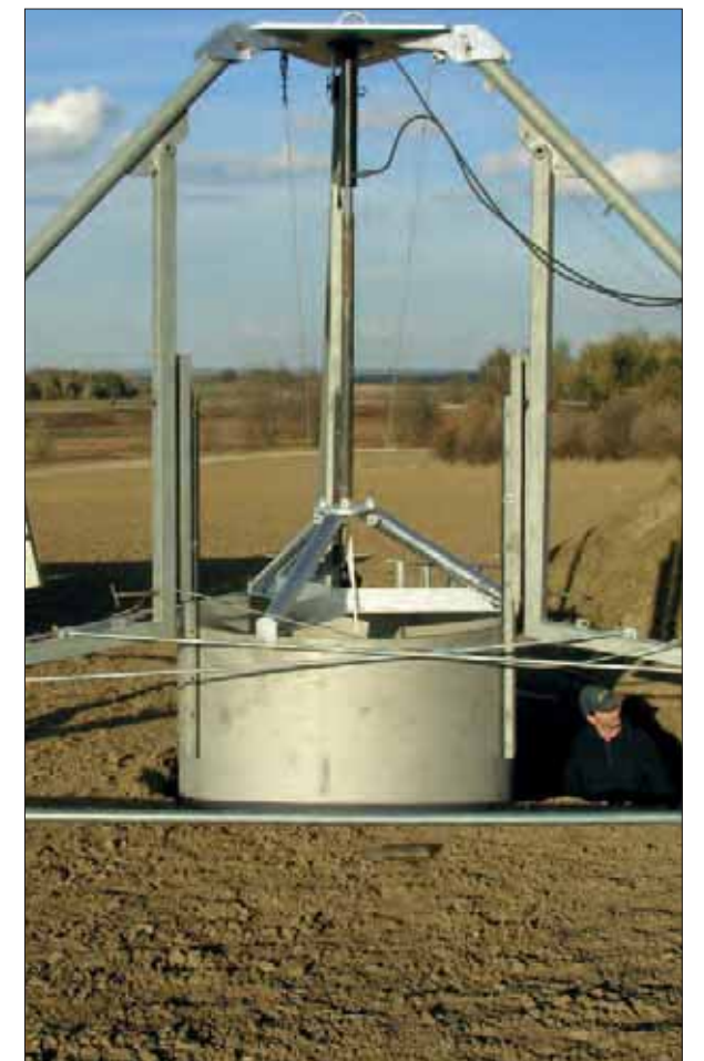
Excavation Technology for a 2 m 2 soil monolith
