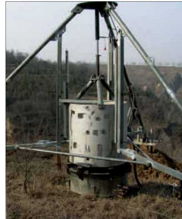
Monolith cutting on a terrace
