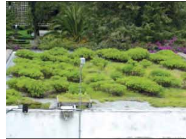
Measuring plots with weighable lysimeters and weatherstation
