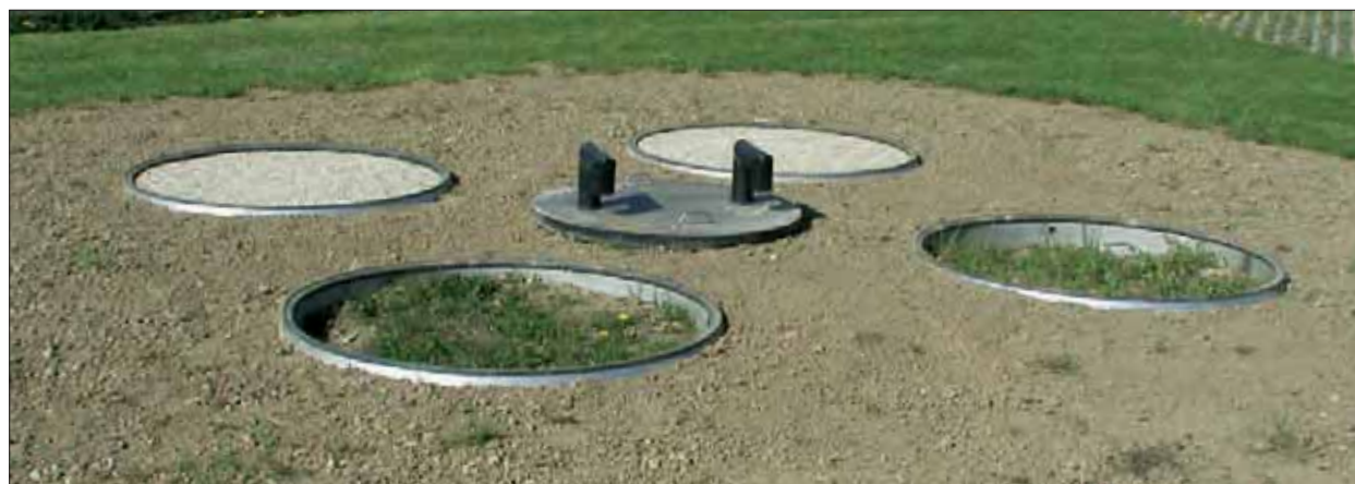
Total view of the containerized lysimeter station with different monolith compositions
