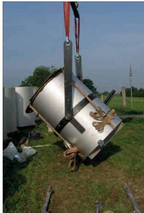
Turning of a 2 m 2 soil monolith
