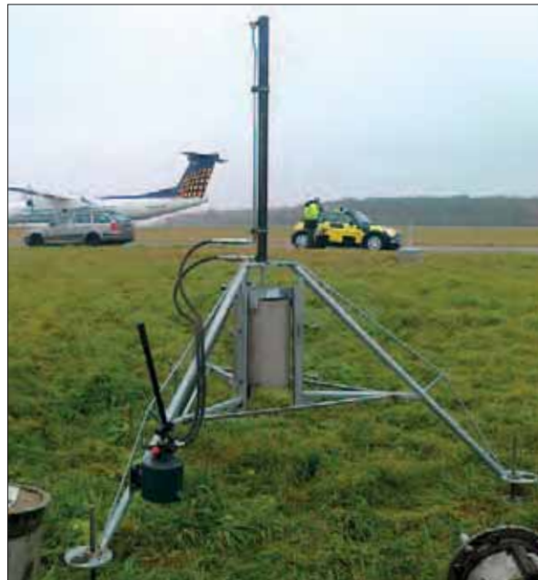
Excavation Technology for a 0,07 m 2 (Ø 30 cm) soil monolith on airport ground
