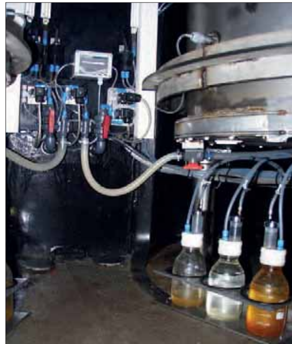
The flow meter in the lysimeter stack
