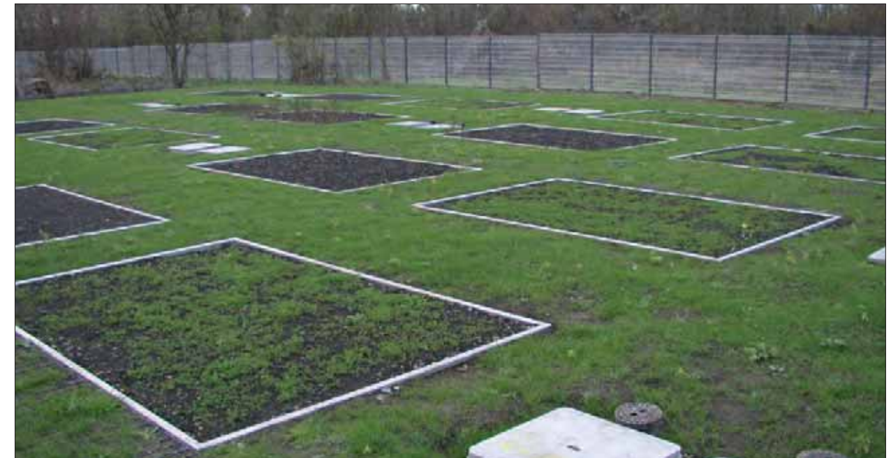
Plate lysimeters with different vegetation the data loggers are stored weatherproof in the grey boxes
