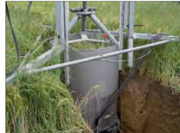
It is also possible to cut soil monoliths with already grown vegetation like here in a barley field.
