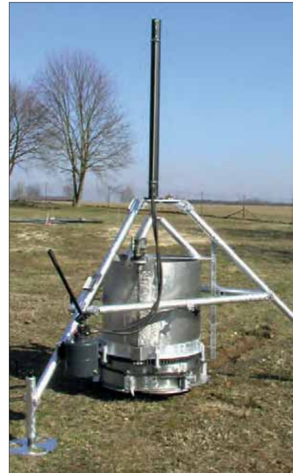
Excavation Technology for a 0,5 m 2 soil monolith
