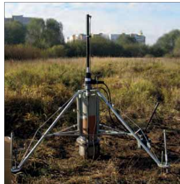
Cutting technology for laboratory soil columns in plastic vessels in use at the Oka floodplain
