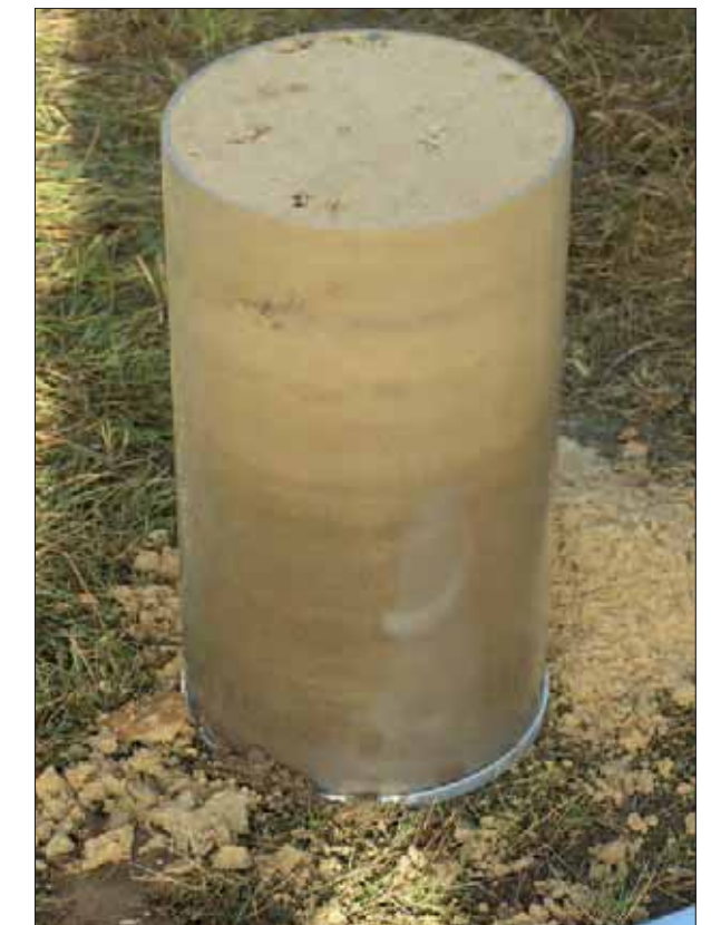
Layered soil in a PMMA cartridge
