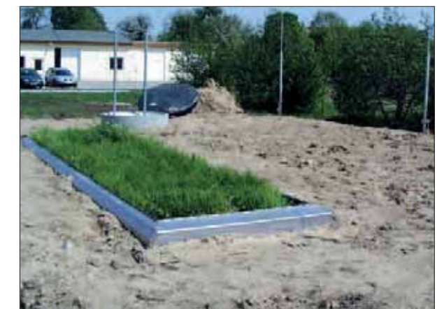
Moor lysimeter directly after installation
