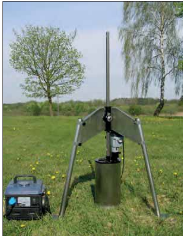
Excavation technology for a 0,03 m 2 (Ø 20 cm) soil monolith
