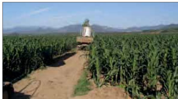
Transport of the soil monolith to the lysimeter station in the maize field
