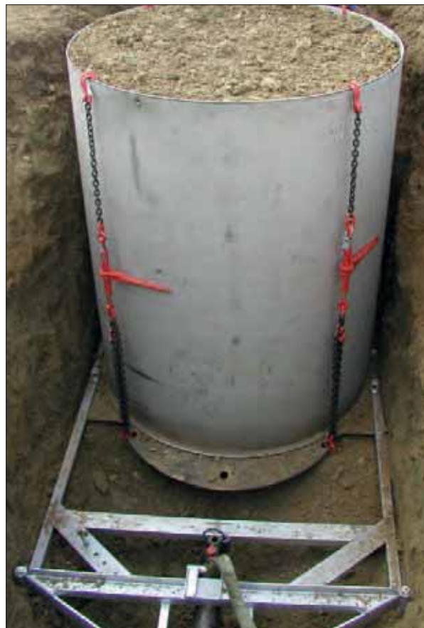
Base cutting with a steel plate of a 2 m 2 soil monolith
