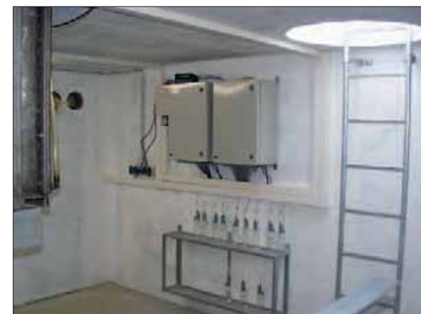
Water sampling technology in the stack
