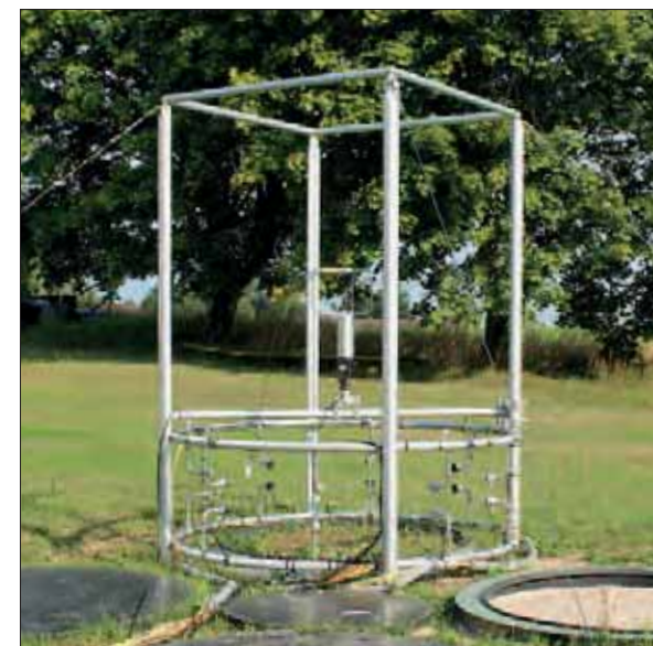
Acoustic chamber on a lysimeter
