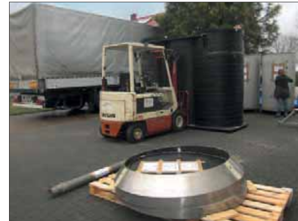
Lysimeter station ready for transport
