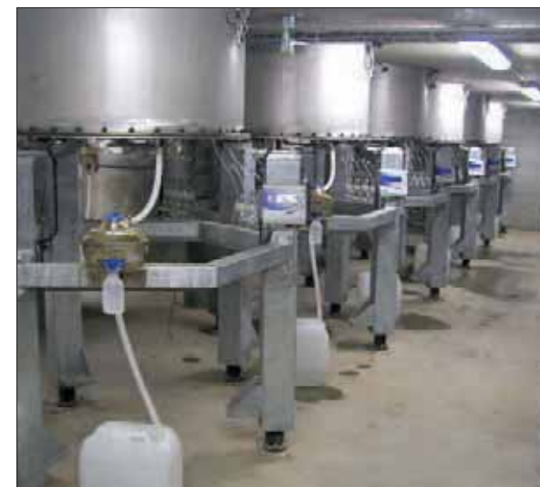
Collecting and counting of seepage water by tipping buckets
