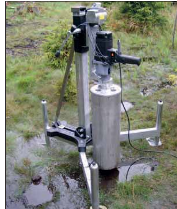
Vertical excavation technique for fen soils
