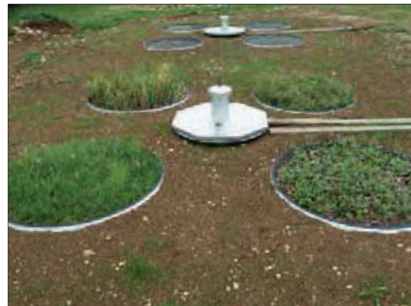
Comparison of lysimeters with vegetation and with clay surface
