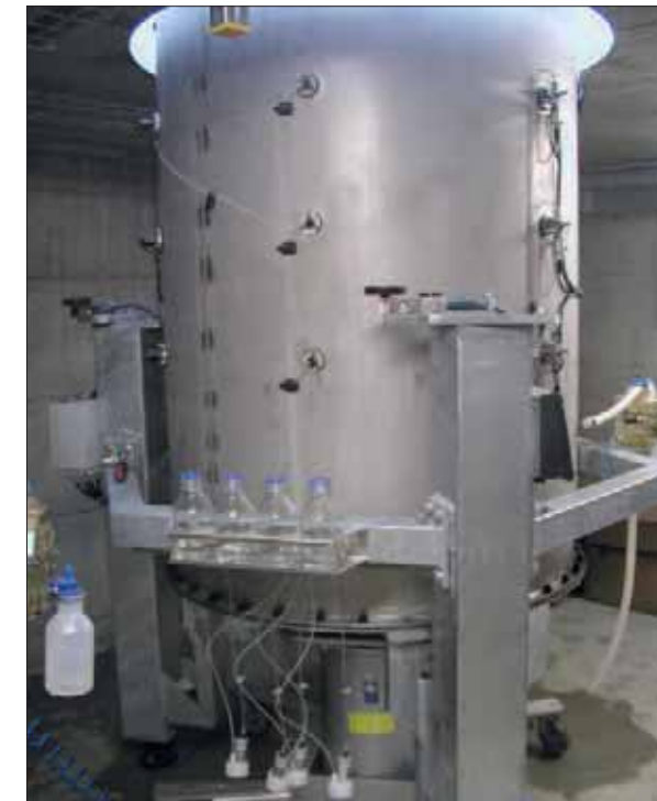
Lysimeter in maintenance position
