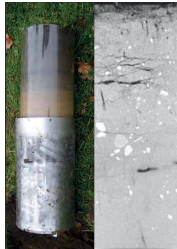
PMMA cartridges make the soil column and its layers visible additionally computer tomography enables to even look inside the soil columns to find cracks or roots
