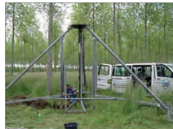
Cutting of a 1 m 2 soil monolith
