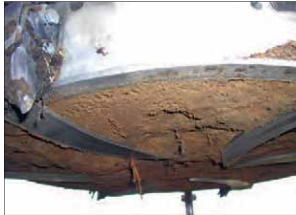
Base cutting with steel fins of a 0,5 m 2 soil monolith
