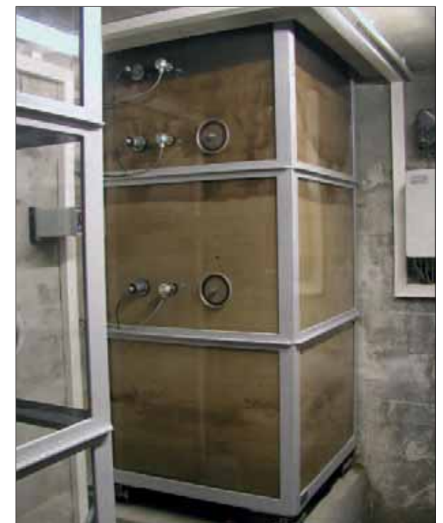
Weighable lysimeter with soil hydraulic sensors
