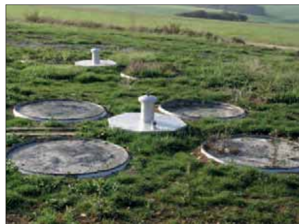
Lysimeters with clay surface after growing of surrounding vegetation
