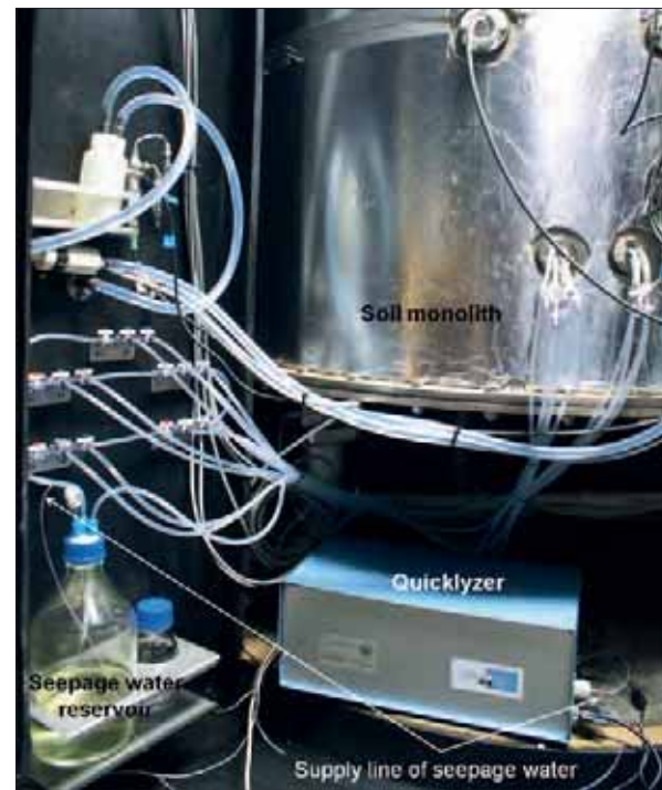
Quicklyzer installed at a lysimeter
