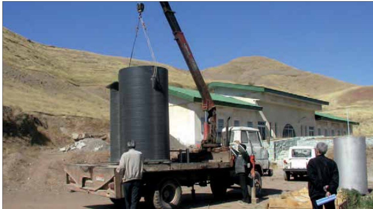
Delivery of the lysimeter equipment at the test site in the Elburz Mountains in Taleghan
