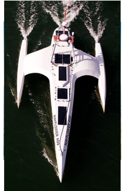
Mayflower Autonomous Ship (MAS) operates without crew using AI to guide it using a range of onboard sensors combined with machine learning (photo courtesy Promare/ IBM)
